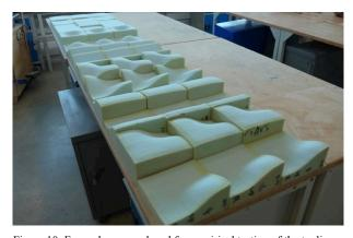
Figure 10: Foam shapes produced for empirical testing of the tooling system's performance, photo: T. Jørgensen, 2014.
