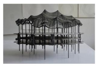
Figure 3: RPT system with glass bowl (upside down) still resting on the pins following the slumping process, photo: T. Jørgensen, 2012.
