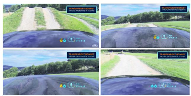
Figure 2: The vision video of 'The Transparent Bonnet system' showing the SUV approaching a hill, prompting the augmented reality (AR) HUD to made the front hood semi transparent while climbing the hill, before it agains turns solid (Land Rover UK 2014a).
