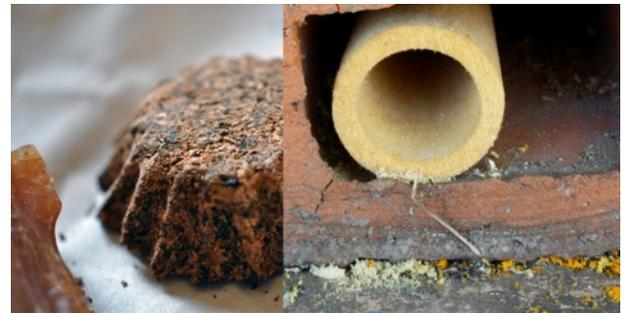
5 – Sample of material experimentation with wood from ‘Palo borracho’ (genus *Chorisia*). On the bottom left it is possible to see part of hardened resin from a native *Acacia* used as binder to make the soft compound material. On the right (photo: Mariano Lucia), it is possible to see the sawdust from the scraping of the inner walls of the MDF cylinder, as well as pollen disseminated while entering and leaving the cylinders.
